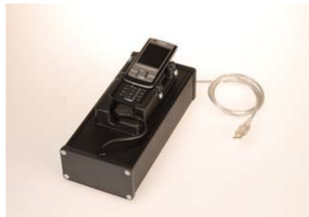
The UEControl tabletop module is especially designed for Drive Tests with 3GMA
